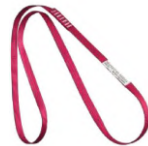
PAT 900 20 mm wide polyester strap anchor point. 22 kN and 6 available lengths: 0.3, 0.6, 0.8, 1.2, 1.5 and 2 m.
