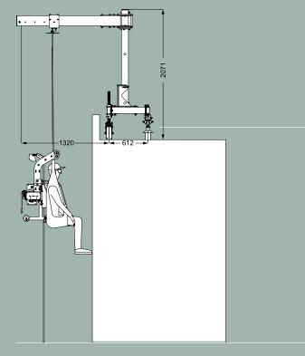
The stability of the trolley is ensured by two wheel boxes taking up the tilting moment thanks to the aluminum Safeaccess rail fixed on posts
