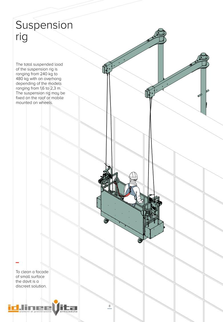
To fix the davit on the roof, a series of sockets are installed along or on the parapet. Several types of sockets are standardised, two sockets on roof slab and one socket on parapet. It can be custom-made upon reques
