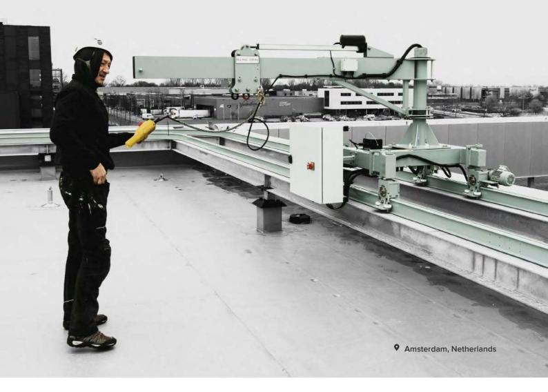
Fallprotec has designed several innovative and compact solutions for facade maintenance equipments. It is thanks to the innovations that integrate the RopeClimber person lifting hoist that a significant reduction in weight of the equipment has been achieved, among which:
