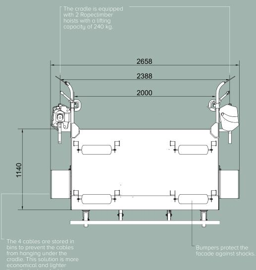
than that using electric reels to store the cables.
