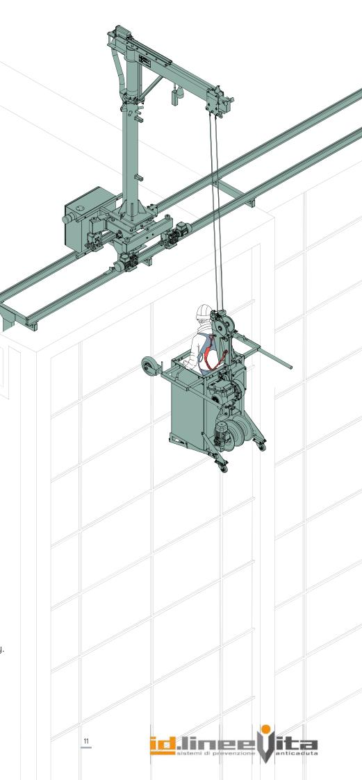
The powered trolley for one man cradle. The trolley is powered by a battery, no need to provide electrical power plugs on the roof, or by main supply. The trolley is controlled from the cradle by an HF transmission.
