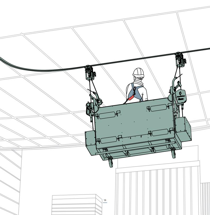
SafeAccess consists of an aluminium rail fixed to the structure of the building by a series of supports and one or two trolleys from which are suspended a cradle or a bosun chair. Installed at the time of construction or on an existing building, it is attached to the facade or to the ceiling for cleaning facades. NAV trolleys are either manual or
