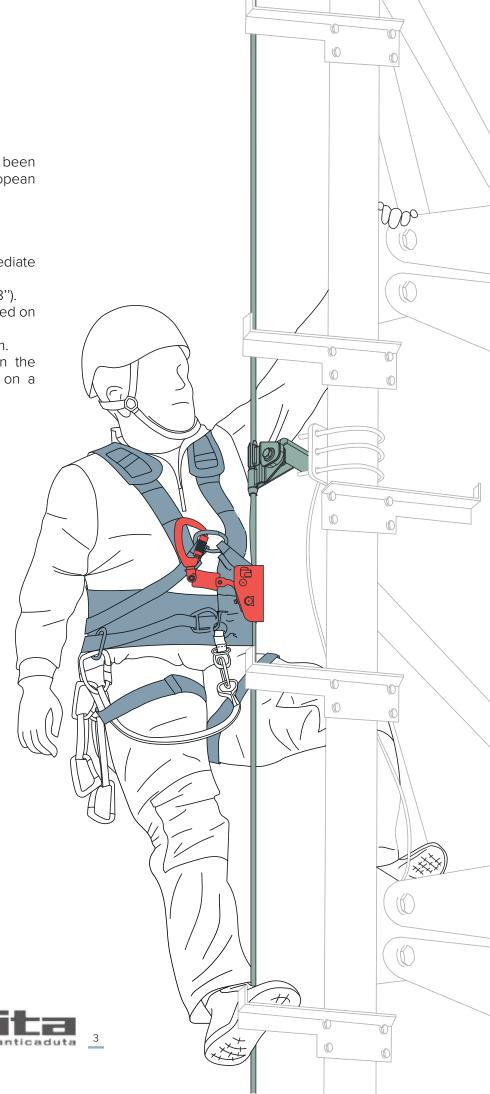
Fallprotec provides a vertical cable lifeline Securope. It can be retrofitted on an existing ladder or structure. Installed without crimping, it comes with an opening glider that allows the user to keep safely connected while being capable to connect to the lifeline at whichever time he wishes. The glider blocks automatically in case of a fall.
