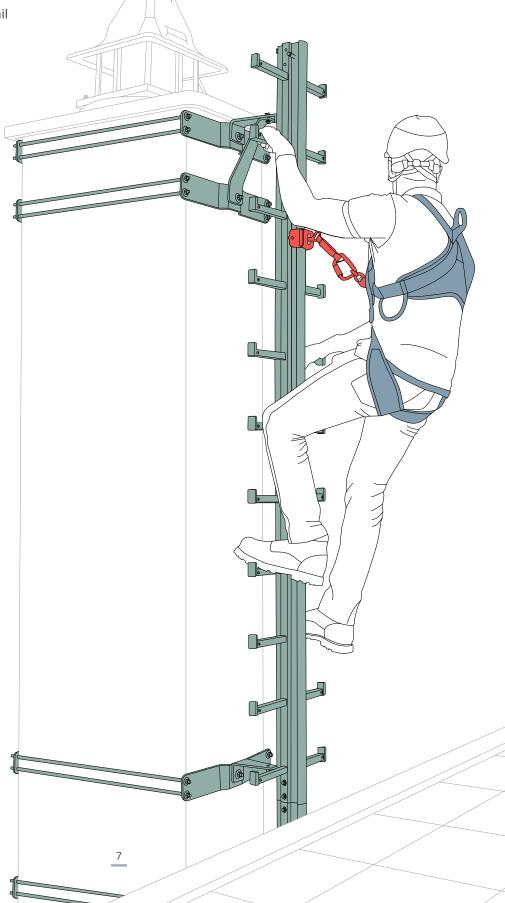
Aluminium fall arrest rail with integrated rungs. High strength profile for fixation on metallic structures or in confined spaces.
